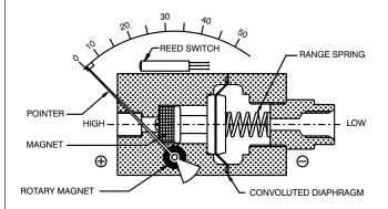
Instrument consists of a convoluted diaphragm to sense the pressure difference. It can withstand maximum operating pressure up to 100 bar for all ranges. If pressure exceeds the rated maximum pressure, "O" rings & diaphragm inside the pressure chamber, will be damaged. If maximum operating pressure is within the allowable limit of 100 bar, but the differential pressure exceeds instrument range, there will be no damage to the instrument. Pointer will only go the extreme right end of the scale.
