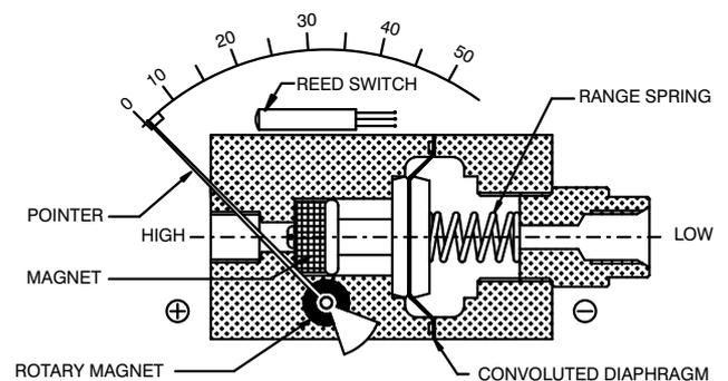
Instrument consists of a convoluted diaphragm to sense the pressure difference. It can withstand maximum operating pressure up to 100 bar for all ranges. If pressure exceeds the rated maximum pressure, "O" rings & diaphragm inside the pressure chamber, will be damaged. If maximum operating pressure is within the allowable limit of 100 bar, but the differential pressure exceeds instrument range, there will be no damage to the instrument. Pointer will only go the extreme right end of the scale.
