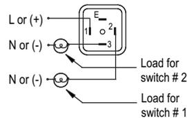
View of plug after removing the socket
