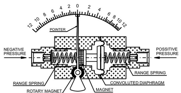
Compound (center zero) instruments consists of a small convoluted diaphragm to sense the pressure difference. It can withstand maximum operating pressure up to 100 bar for all ranges.
