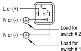
View of plug after removing the socket
