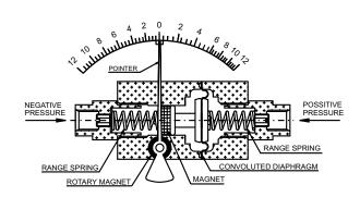
Compound (center zero) instruments consists of a small convoluted diaphragm to sense the pressure difference. It can withstand maximum operating pressure up to 100 barfor all ranges.
