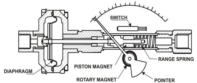
If maximum operating pressure is within the maximum specified pressure for the instruments, but the differential pressure exceeds instrument range, there will be no damage to the instrument. Pointer will only go to the extreme right end of the scale.
