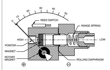
Instrument consists of a rolling diaphragm to sense the pressure difference. It can withstand maximum operating pressure up to 200 bar for all ranges. If pressure exceeds the rated maximum pressure, "O" rings & diaphragm inside the pressure chamber, will be damaged. If maximum operating pressure is within the allowable limit of 200 bar, but the differential pressure exceeds instrument range, there will be no damage to the instrument. Pointer will only go the extreme right end of the scale.
