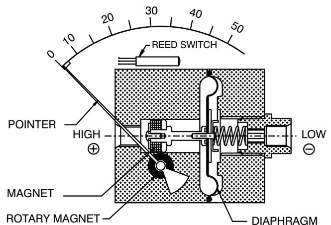
If pressure exceeds the rated maximum pressure, "O" rings & diaphragm inside the pressure chamber, will be damaged. If maximum operating pressure is within the allowable limit of 35 bar, but the differential pressure exceeds instrument range, there will be no damage to the instrument. Pointer will only go the extreme right end of the scale.
