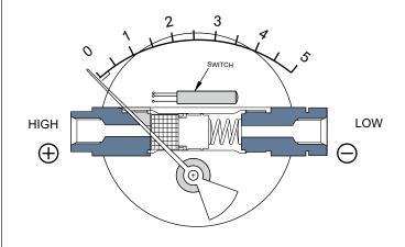
If pressure exceeds the rated maximum pressure, "O" rings used on male connectors, and the seal inside the pressure chamber, will be damaged. If maximum operating pressure is within the allowable limit of 400 bar, but the differential pressure exceeds instrument range, there will be no damage to the instrument. Pointer will only go to the extreme right end of the scale.
